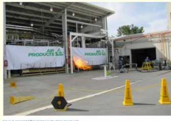
Figure 4: Horizontal flare testing at the clean energy lab.
