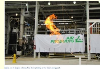
Figure 3.6: 45-degree release flare during testing at the clean energy lab.
