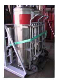
ENSURE PLC remains upright & secured by using a restraint-ratchet belt
