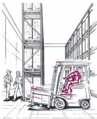
Load shall be kept close to the forklift mast and tilted backwards
