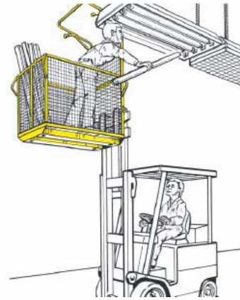
The lifting of people is allowed only with suitable equipment provided in the user manual of forklift
