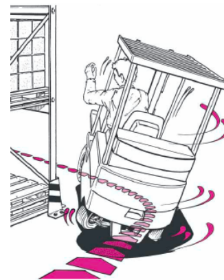
In case of forklift overturning, do not leave the forklift but: Remain sit hold onto the steering wheel well push your feet on forklift floor tilt the side opposite to that of overturning
