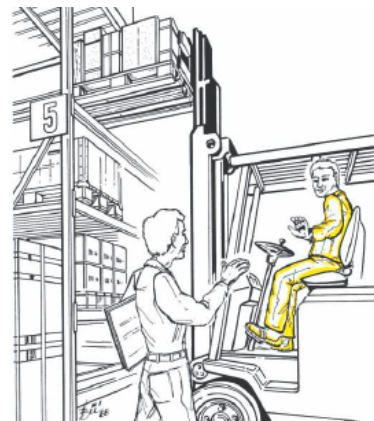
Check that nobody is near the raised load
