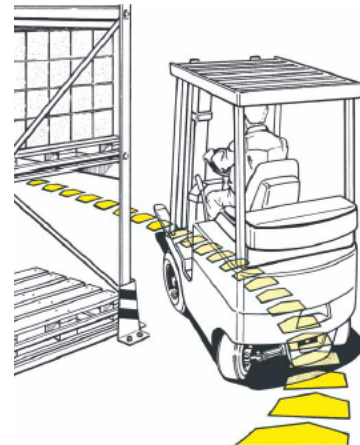
Drive round curves at low speed, Accelerate with caution
