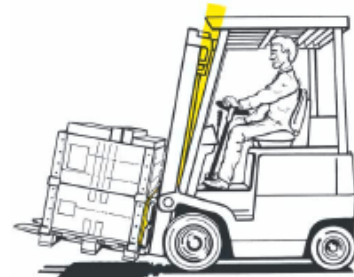
Load shall be kept close to the forklift mast and tilted backwards
