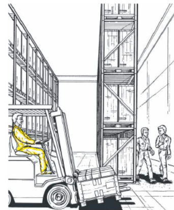
Load shall be kept close to the forklift mast and tilted backwards
