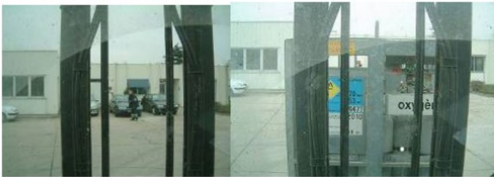
Example of bad visibility from the forklift driver's seat
