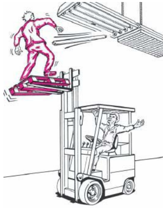
The lifting of people is allowed only with suitable equipment provided in the user manual of forklift
