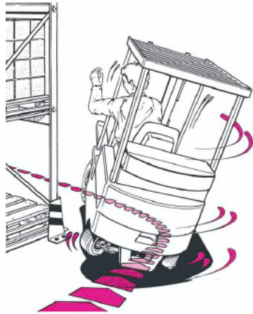
Drive round curves at low speed, Accelerate with caution
