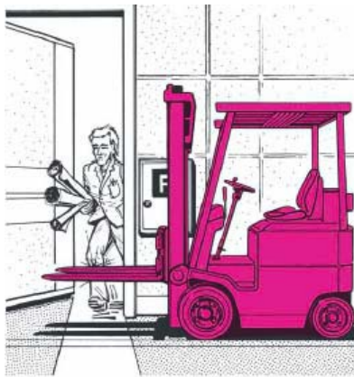
Park forklift in the proper way, fork low and not in front of door or emergency exit
