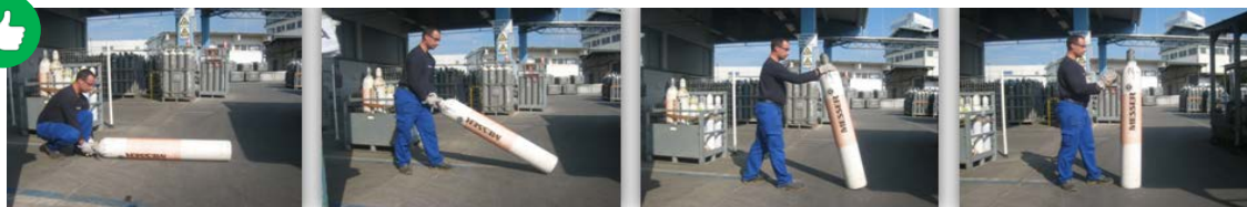
Thao tác nâng chai đúng / Correct cylinder lifting operation
