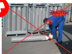
Thao tác nâng chai sai / Incorrect cylinder lifting operation
