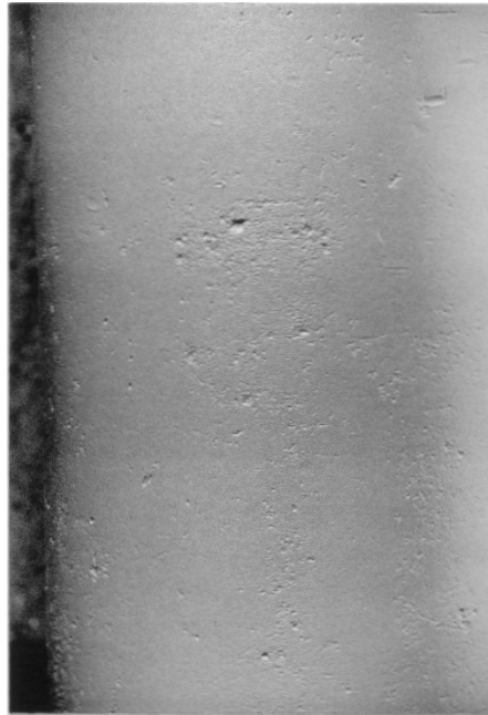
Figure 8—General corrosion with isolated pitting on cylinder sidewall
