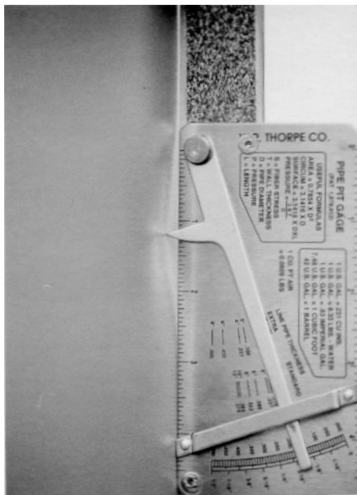
Figure 10—Measuring the length and depth of typical dent
